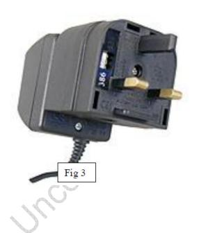
Insert the VDE Plug as shown and tighten the screw on the base to 0.6Nm. (6.12 Kgf.cm)
